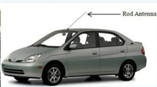
Fig. 2 Rod antenna mounted on car
